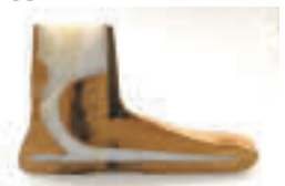
Figure 2. MIT drip irrigation emitter design with novel features to reduce pumping energy and potentially prevent clogging.
