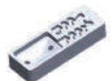
Figure 2. MIT drip irrigation emitter design with novel features to reduce pumping energy and potentially prevent clogging.
